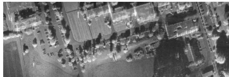
*SAR image of the compound of Fraunhofer FHR measured with MIRANDA-94 with 94 GHz operational frequency and 2 GHz bandwidth. The resulting image resolution is 7.5 cm.*
