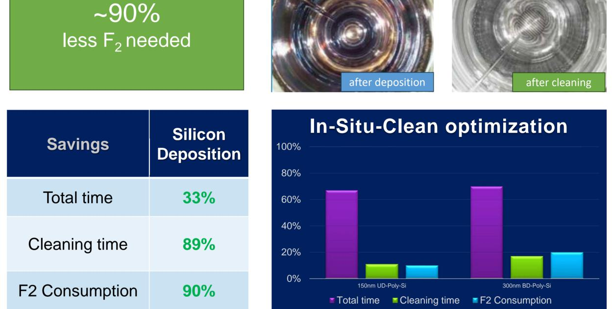
Thermal thin film deposition of Polysilicon layers by Low Pressure Chemical Vapour Deposition (LPCVD) on silicon substrates followed by in-situ dry clean of reactor parts using Fluorine gas ( $F_2$ ).
