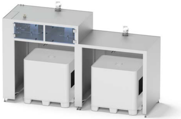
Original Slurry Supply System
