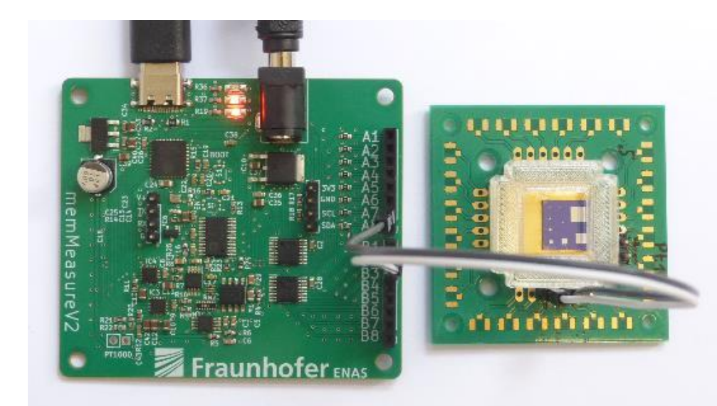
MemMeasure board for transient characterization memristive components for neuromorphic circuits
