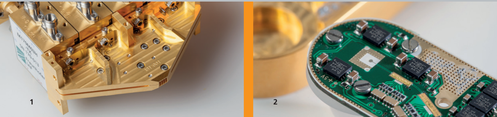
1 The 4-channel Rx/Tx module allows THz technologies at 300 GHz for wireless networks beyond 5G.
